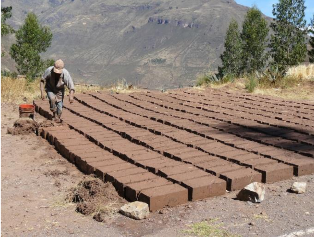
Figure 4-18 – Adobe bricks being dried in the sun.
